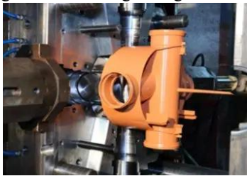
Sewage Chamber Mould
