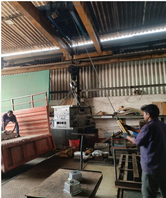
Unloading Mould Machine
